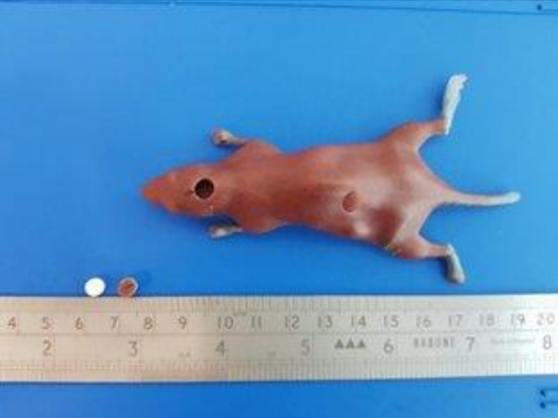
Figure 7. Details of the small animal phantom with alanine detector
