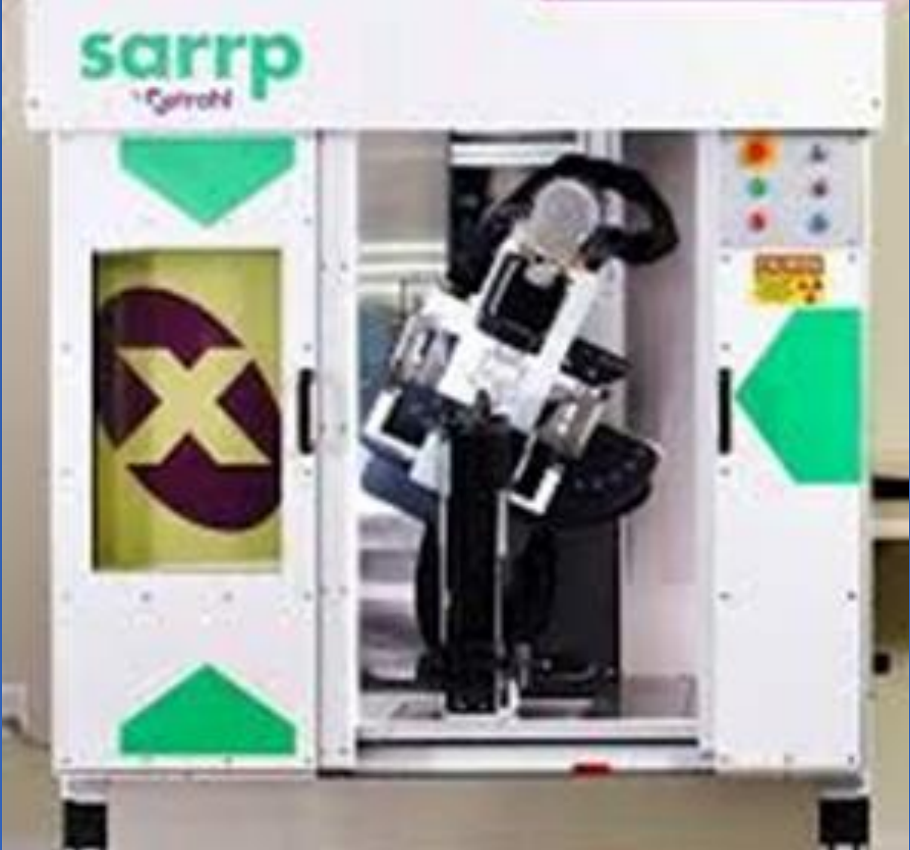
Figure 1. Image of a Small Animal Radiation Research Platform (SARRP)
